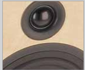
25MM NITRO-URETHANE LAYER DAMPED WOVEN POLYESTER DOME, SHIELDED NEODYMIUM MAGNET ASSEMBLY.
